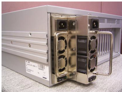
Figure 3.12: Replacing the 400W redundant power supply module
