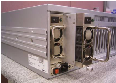
Figure 3.11: Replacing the 300W redundant power supply module
